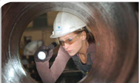
Visual inspection for surface cracks
