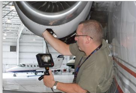
Inspection of Aircraft using Fiberscope
