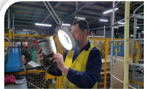
Direct visual inspection of welded parts
