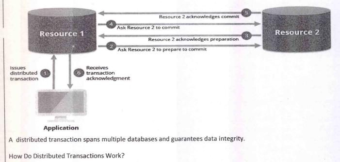
Distributed transactions have the same processing completion requirements as regular database transactions, but they must be managed across multiple resources, making them more challenging to implement for database developers. The multiple resources add more points of failure, such as the separate software systems that run the resources (e.g., the
