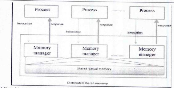
Distributed Shared Memory (DSM) is an abstraction that allows distributed systems to share a single memory space among multiple nodes. This abstraction enables processes on different machines to access shared data as if they were on the same physical memory. DSM simplifies the development of distributed applications by providing a shared memory model, abstracting away the complexities of message passing.
