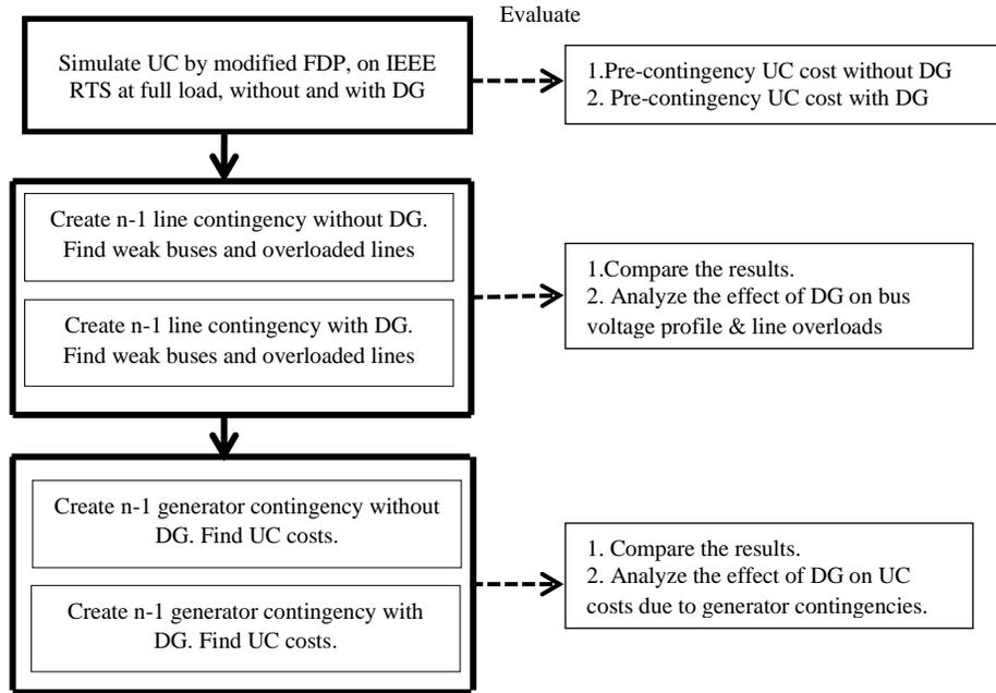
**FIGURE 1.** Block diagram of  $n-1$  generator contingency based UC
