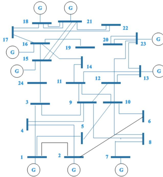
FIGURE 2. Single Line Diagram of modified IEEE RTS
