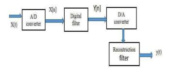
Figure-1: A continuous-time signal filtering system, made for a digital filter
