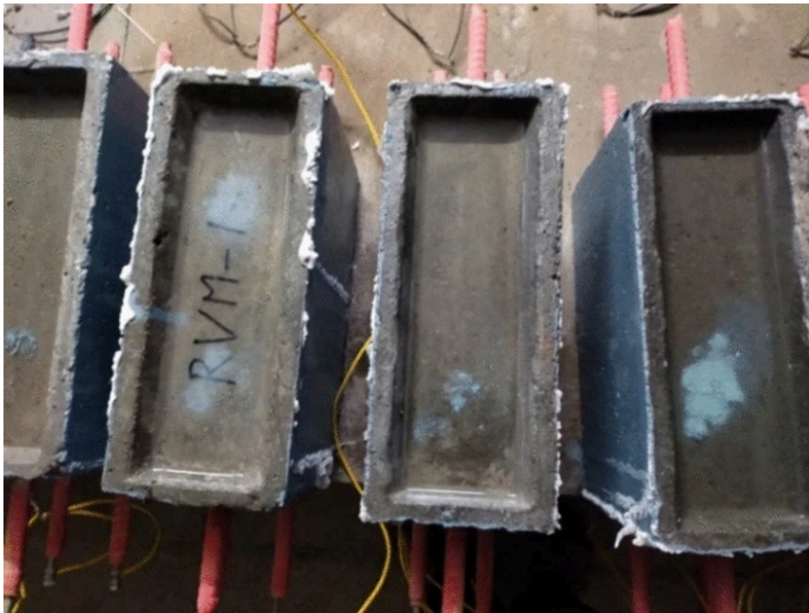
Corrosion specimens with ponding facility
