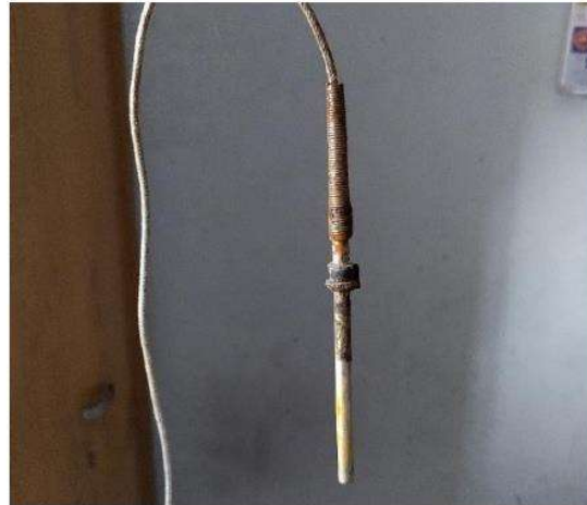
Figure 2: Damaged RTD due to corrosion
