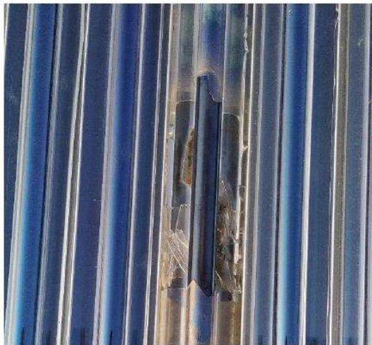
Figure 1: Damaged tubes of ET-CPC solar field
