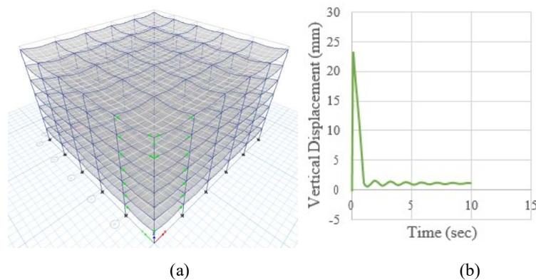
**Fig. 7.** Case 4: Corner column removal, peripheral beam 300 x 500 mm, grid size 6m x 6m (a) Hinges formed in the structure; (b) Vertical Deflection at column removal location
