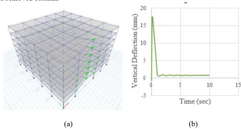
**Fig. 3.** Case 1: Middle column removal, peripheral beam 300 x 500 mm, grid size 6m x 6m (a) Hinges formed in the structure; (b) Vertical deflection at the column removal location
