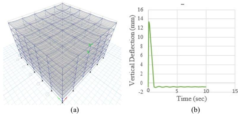
**Fig. 4.** Case 2: Middle column removal, peripheral beam 300 x 600 mm, grid size 6m x 6m (a) Hinges formed in the structure; (b) Vertical deflection at the column removal location
