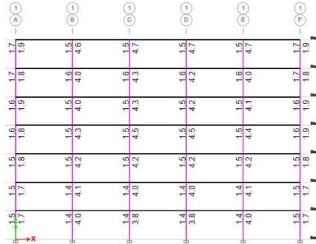
**Fig. 5.** Column-Beam capacity ratios for peripheral beam sizes are 300 x 600 mm, grid size 6m x 6m
