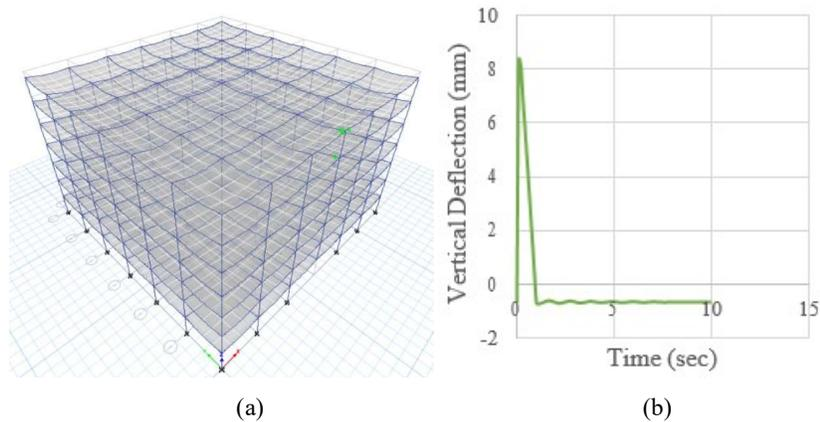
**Fig. 6.** Case 3: Middle column removal, peripheral beam 300 x 500 mm, grid size 5m x 5m (a) Hinges formed in the structure; (b) Vertical Deflection at the column removal location
