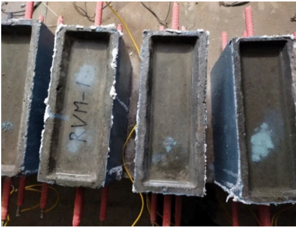
Corrosion specimens with ponding facility
