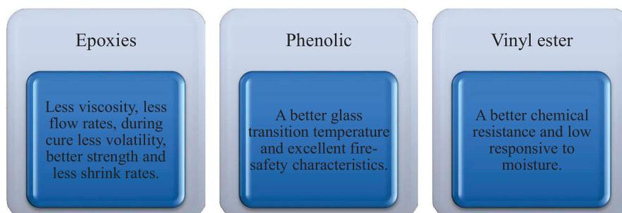
Figure 1.1 Classification of Thermo-set Polymers.
