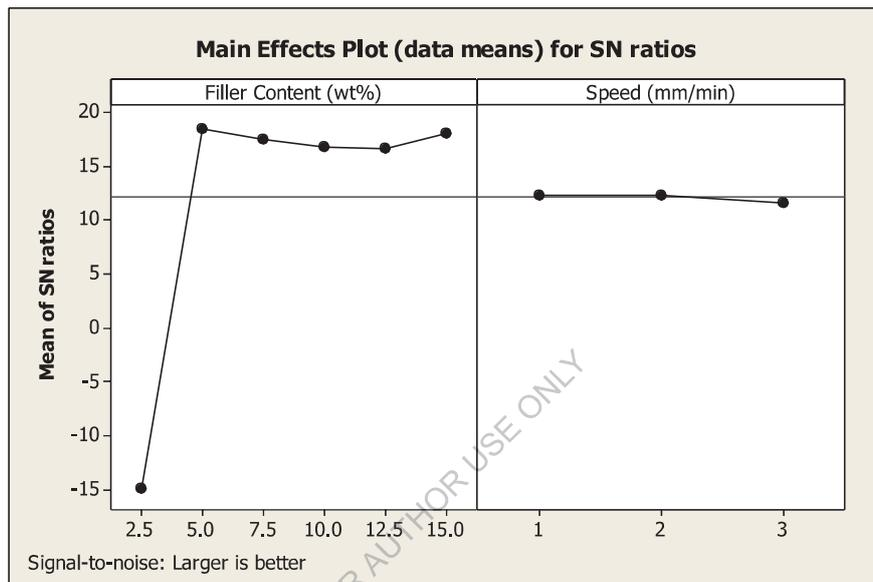
Figure 5.3 Main effects plot for S/N ratio on different percentage of weight of CSP/WSP epoxy based composites in flexural load.
