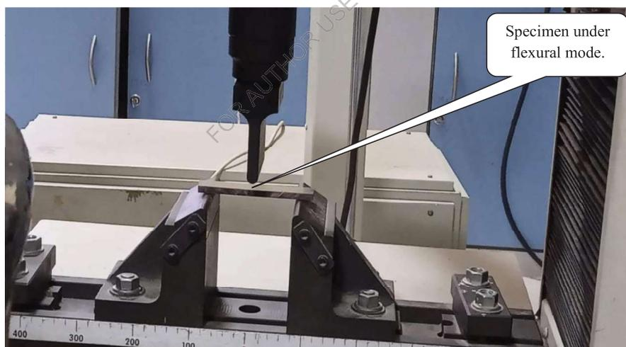
Figure 3.17 Specimen under Flexural Mode (Tinius Olsen Made in USA)
