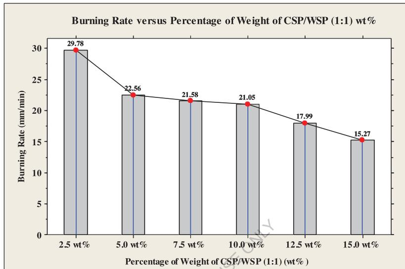
Figure 4.7 Comparison of burning rate of different percentage of weight of CSP/WSP (1:1) particulates reinforced epoxy based composites.
