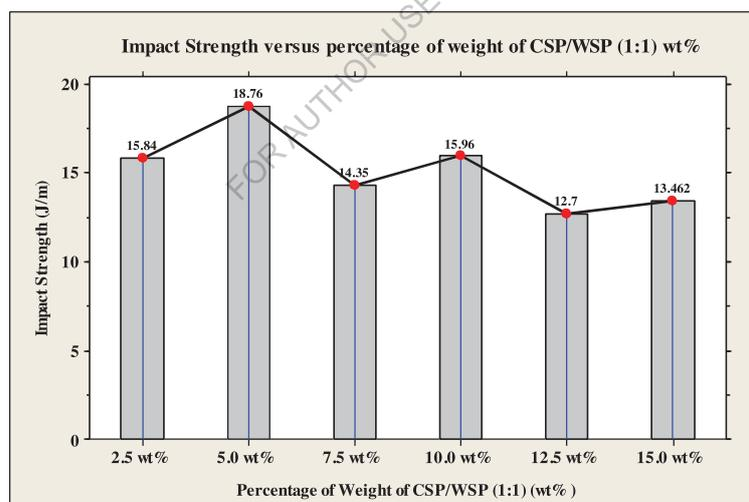
Figure 4.8 Comparison of impact strength of different percentage of weight of CSP/WSP (1:1) particulates reinforced epoxy based composites.
