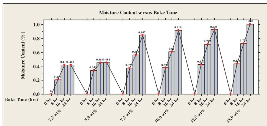
Figure 4.2 Comparison of moisture content of different percentage of weight of CSP/WSP (1:1) particulates reinforced epoxy based composites.
