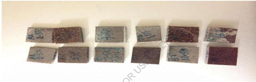
Figure 3.12 Specimens for Thickness Swelling Test.
