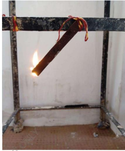
Figure 3.15 (b) Specimens for Flammability Test During Burning.
