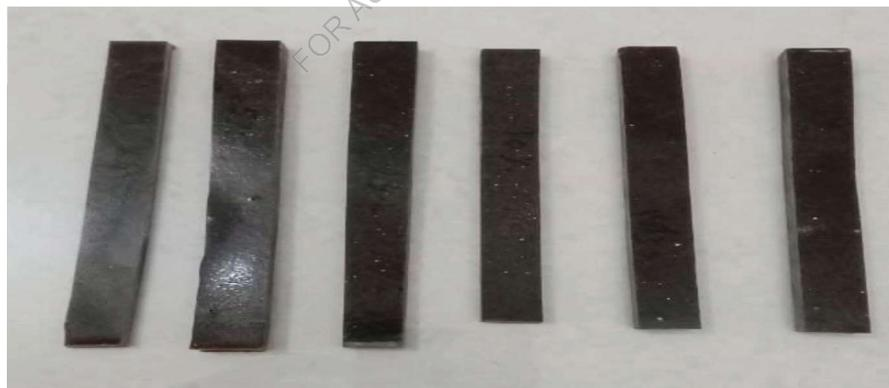
Figure 3.14 Specimens for Flammability Test.
