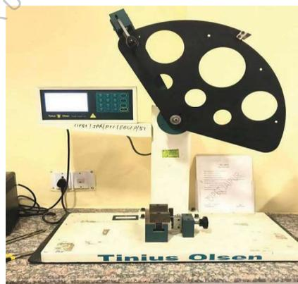
Figure 3.20 Specimen under Impact Mode on Model IT 504 Plastic Impact (Tinius Olsen Made in USA) [Department of Chemical and Petrochemicals at CIPET, Jaipur].
