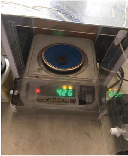
Figure 3.9 (a) Weighing of Specimen in Air
