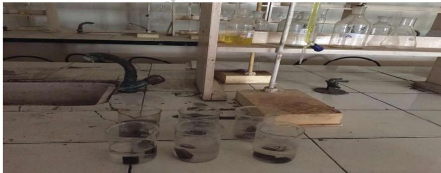
Figure 3.13 Soaking up of Specimen in Tap Water for Linear Swelling Test [RCERT, Jaipur].
