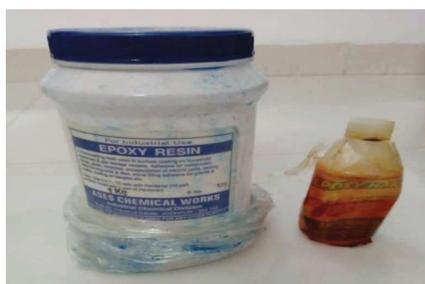
Figure 3.2 Epoxy Resin (LY 556) with Hardener (HY951).
