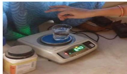
Figure 3.7 (b) Weighing of Specimens in Distilled Water [RCERT, Jaipur].
