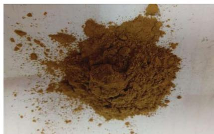
Figure 3.4 (b) Coconut Shell Particular (Mesh 210).
