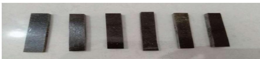
Figure 3.18 Specimens for Impact Test.
