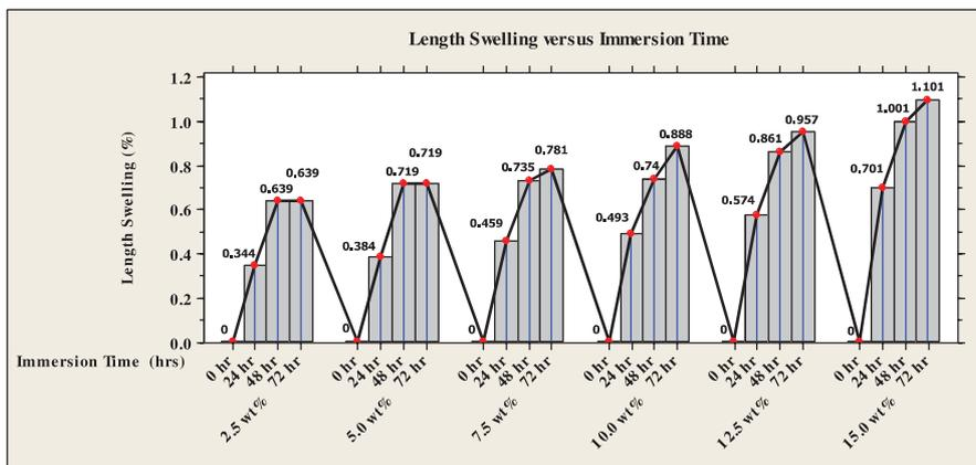
Figure 4.5 Comparison of length swelling of different percentage of weight of CSP/WSP (1:1) particulates reinforced epoxy based composites.
