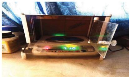
Figure 3.7 (a) Weighing of Specimen in Air [RCERT, Jaipur].
