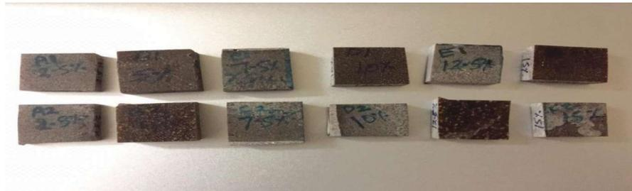
Figure 3.10 Specimens for Water Absorption Test.
