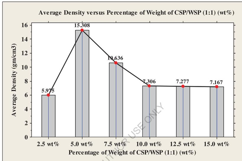
Figure 4.1 Comparison of density of different percentage of weight of CSP/WSP (1:1) particulates reinforced epoxy based composites.
