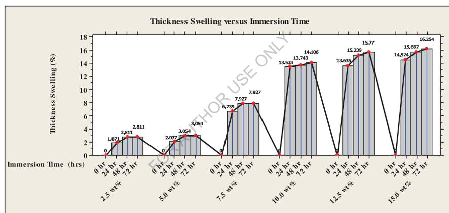
Figure 4.4 Comparison of thickness swelling of different percentage of weight of CSP/WSP (1:1) particulates reinforced epoxy based composites.
