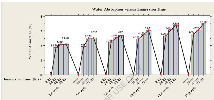
Figure 4.3 Comparison of water absorption of different percentage of weight of CSP/WSP (1:1) particulates reinforced epoxy based composites.
