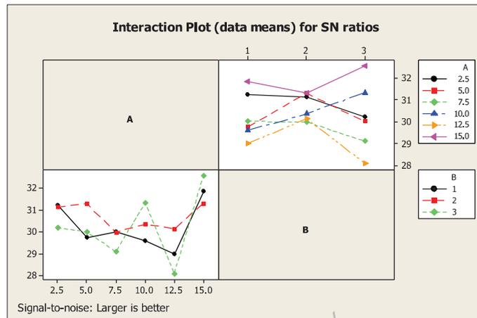
Figure 5.2 Interaction plot for S/N ratio on different percentage of weight of CSP/WSP epoxy based composites in flexural strength.
