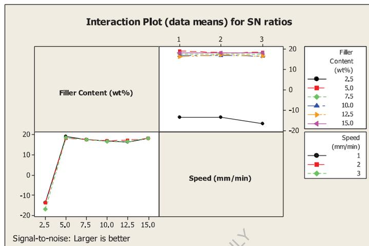
Figure 5.4 Interaction plot for S/N ratio on different percentage of weight of CSP/WSP epoxy based composites in flexural load.
