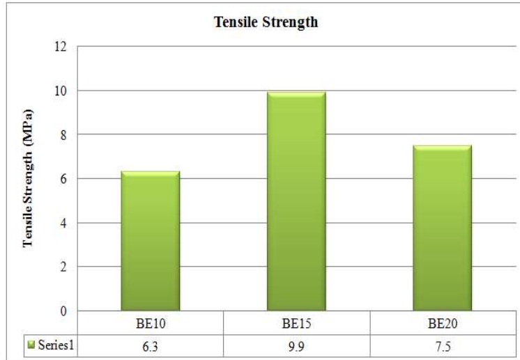
FIG. 5. Comparison of Tensile strength using different wt.% of Banana Fiber
