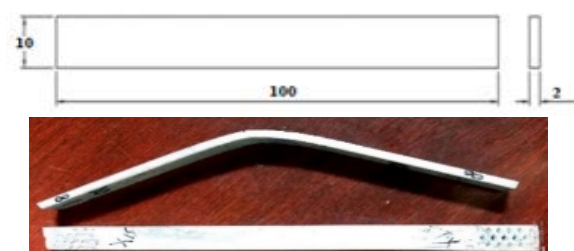
Fig.3: Flexural test specimen
