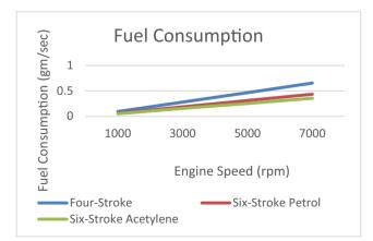
Fig. 13 Fuel consumption vs engine speed
