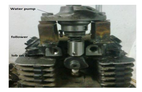
**Fig. 12** The modified water injector pump arrangement
