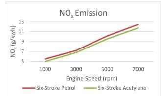
Fig. 18  $NO_x$  emission vs engine speed
