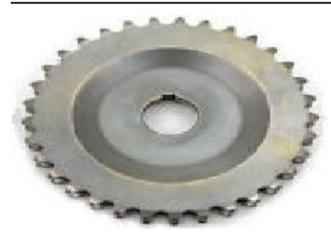
Fig. 9 The modified sprocket with 33 teeth
