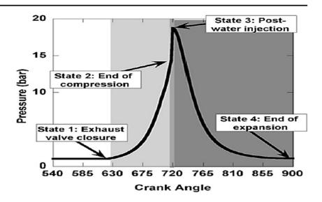
higher as compared to the four-stroke engine. Extra expansion stroke helps in converting more energy into useful work.
