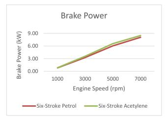
Fig. 14 Brake power vs engine speed
