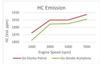
Fig. 17 HC emission vs engine speed
