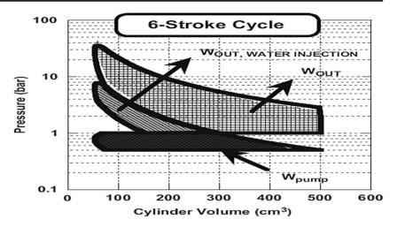
stroke engine to investigate its performance with water injection. It was reported that the increased efficiency of six-stroke cycle engine is due to heat recovery from engine exhaust (in the cylinder) and from coolant (to heat water prior to injection). The six-stroke engine is an efficient mean of in-cylinder waste heat recovery with water injection in the fourth stroke.
