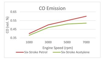
Fig. 16 CO emission vs engine speed
