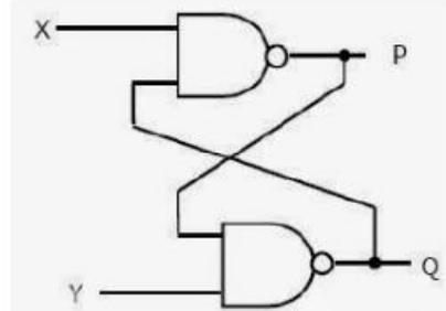
**Q3.** When the race around condition will occur in the circuit given
