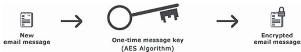
FIGURE 13–7 Encryption of data using Advanced Encryption Standard method.
