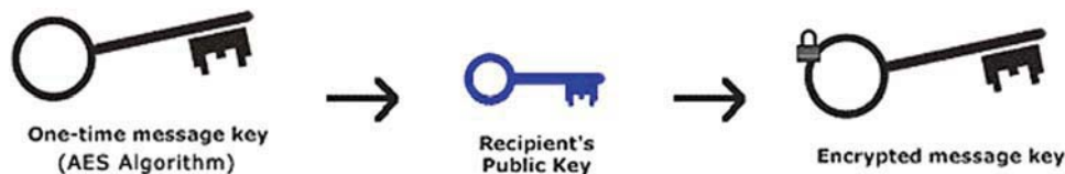
FIGURE 13–8 Encryption of random key using the RSA method.
