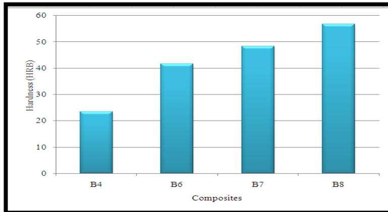
**Figure 8: Hardness of unfilled banana fibre**
