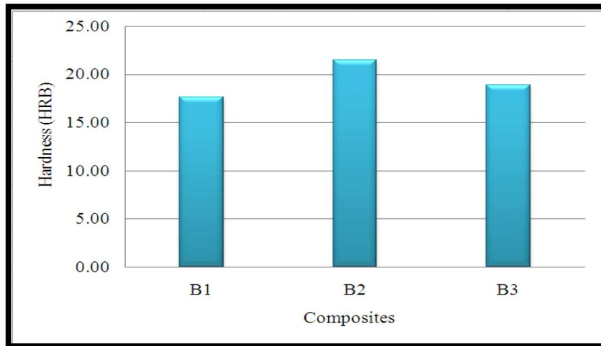
**Fig. 4 Impact of fibre length on hardness**
