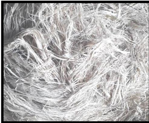
**Fig 1(a):** Pictorial view of uncut nonwoven banana fibre
