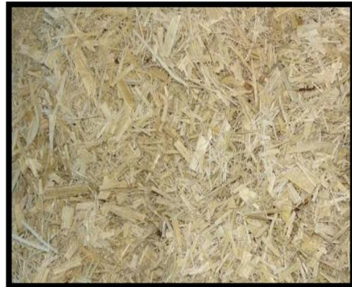
**Fig 1(b):** Pictorial view of chopped nonwoven banana fibre
