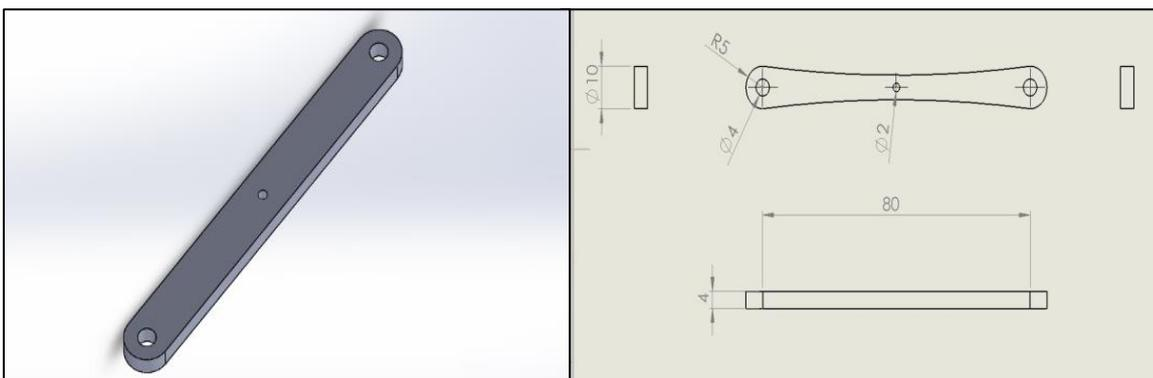
Fig. 6 : Connecting Shaft (model view with dimensions )
