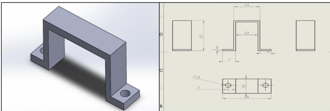
Fig. 5 : Clamp (model view with dimensions )
