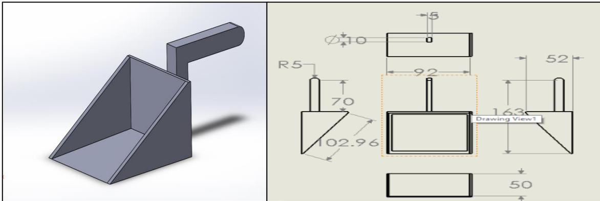
Fig. 4 : Holder (model view with dimensions )
