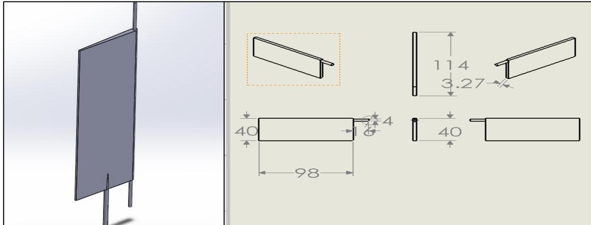
Fig. 7 : Wings (model view with dimensions )
