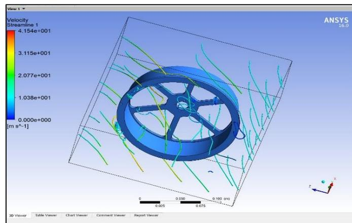
Fig. 11 : Front case simulation for counter air pressure by the chassis
