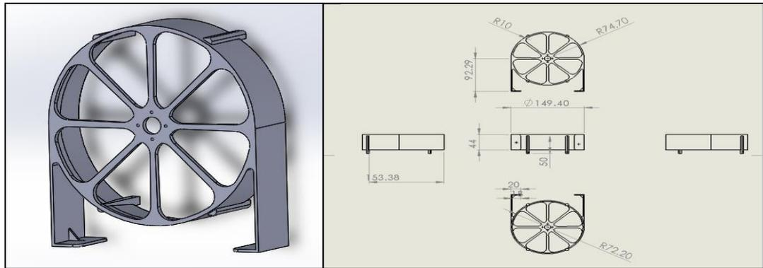
Fig. 3 : Back Case (model view with dimensions )
