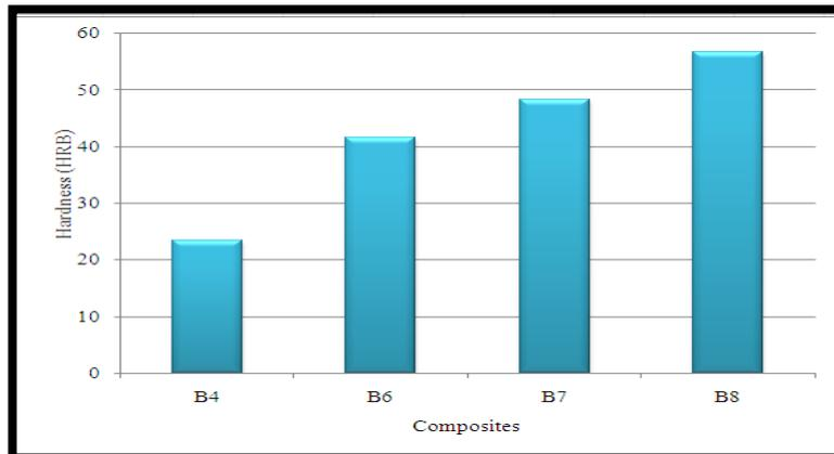
**Figure 8: Hardness of unfilled banana fibre**
