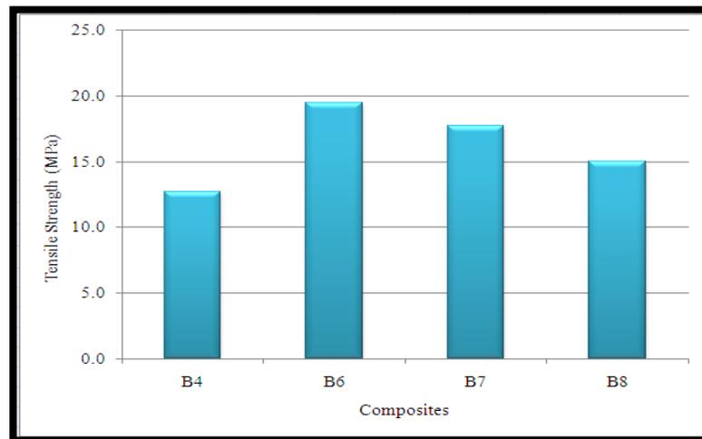
**Fig. 7 Impact of filler loading on tensile strength**
