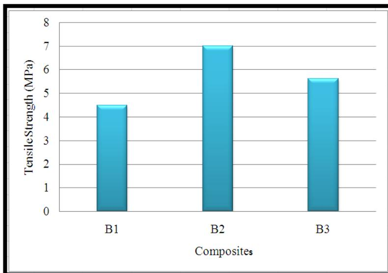
**Fig. 3** Impact of fibre length on tensile strength
