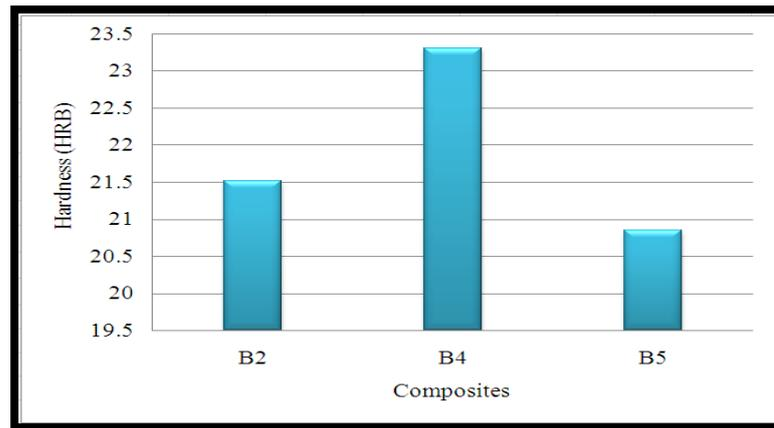
**Fig. 6 Impact of fibre loading on Hardness**
