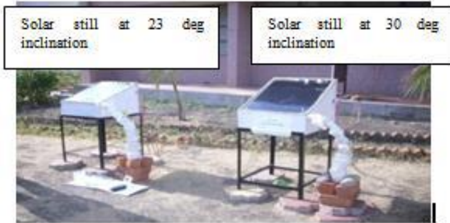
Fig. 10 Solar still at different inclined angles [10]
