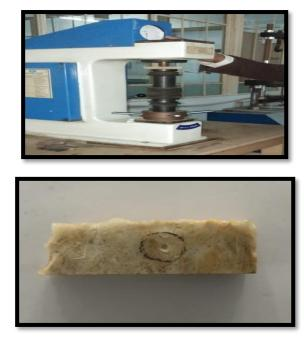
Fig 2(a): Hardness tester (b): Specimen after the measurement of hardness
