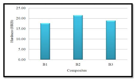
Fig. 4 Impact of fibre length on hardness
