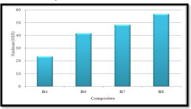
Figure 8: Hardness of unfilled banana fibre
