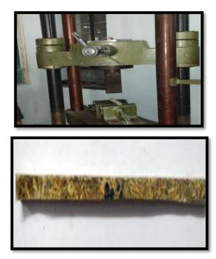
Fig 3(a): Universal testing machine for tensile (b): Test specimen for tensile test
