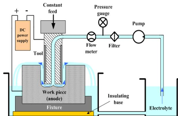
**Fig.1.** Working principle of ECM [3]
