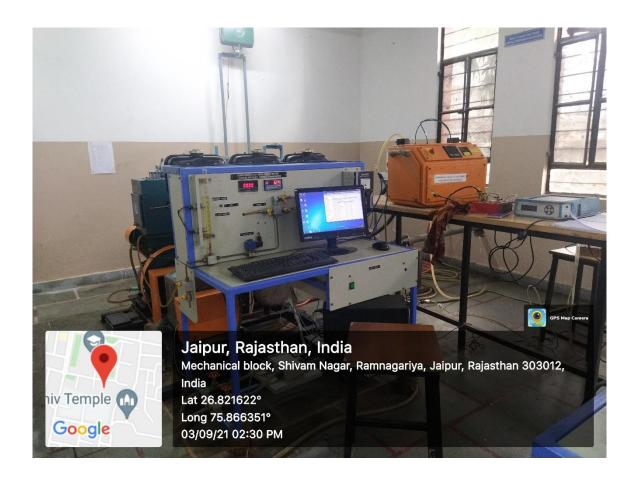
**Equipment Name: Computerised Variable Compression Ratio Diesel Engine**
