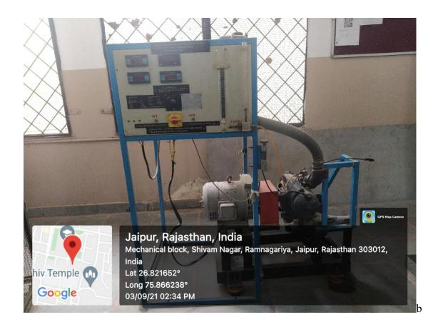
**Equipment Name: Two stroke Motoring Test**
