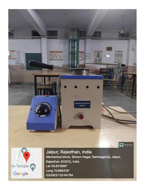
**Equipment Name: CLEAVELAND Flash & Fire Point Apparatus**
