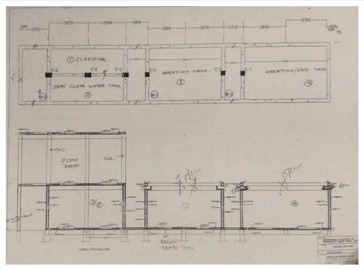
Architecture of Waste Water Recycling Tank\_1
